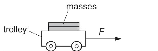
Different masses are placed on the trolley, and acceleration is measured.
